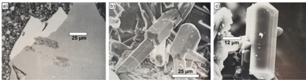
**Figure 7.** (a) SEM photograph of Apollo 10 basalt (10047): fluorapatite in pyroxferrite, in contact with ilmenite. Upper left portion is epoxy; (b) SEM photograph of apatite crystal in Apollo 14 breccia vug; (c) SEM photograph of doubly terminated apatite crystal in Apollo 14 breccia vug. All images from [95].
