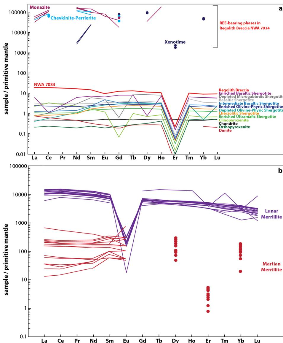
**Figure 8.** (a) Summary of the REE characteristics of martian samples including the recently discovered regolith breccia, NWA 7034 and its REE-bearing phases. All data is available through the Martian Meteorite Compendium [177]. NWA 7034 data from [176]; (b) Comparison of lunar and martian merrillite. Data sources: [116,178].
